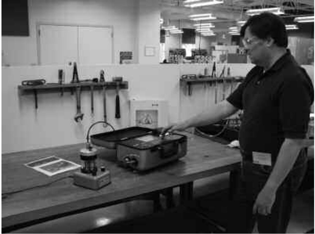
Participants in Eaton's Systemic Contamination Control course learn how to determine the cleanliness of a hydraulic system using the Eaton Target-Pro portable particle counter.
