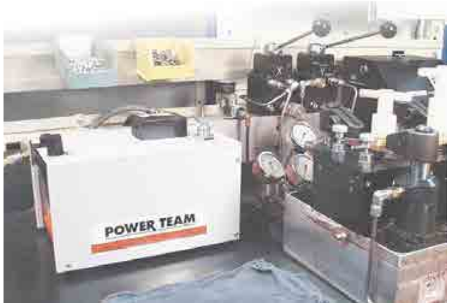
The PA60 used in a workholding environment.
